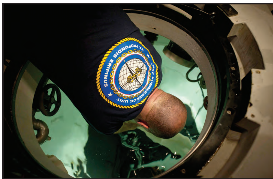
Chief Navy Diver Cory Hall prepares hoses for dewatering inside a sealed chamber connecting the Chilean navy submarine CS Carrera (SS 22) to a pressurized rescue module. (U.S. Navy photo by Karolina A. Martinez/Released)
